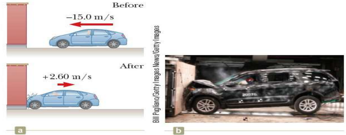
Figure 9.5 (Example 9.3) (a) This car's momentum changes as a result of its collision with the wall. (b) In a crash test, much of the car's initial kinetic energy is transformed into energy associated with the damage to the car.
