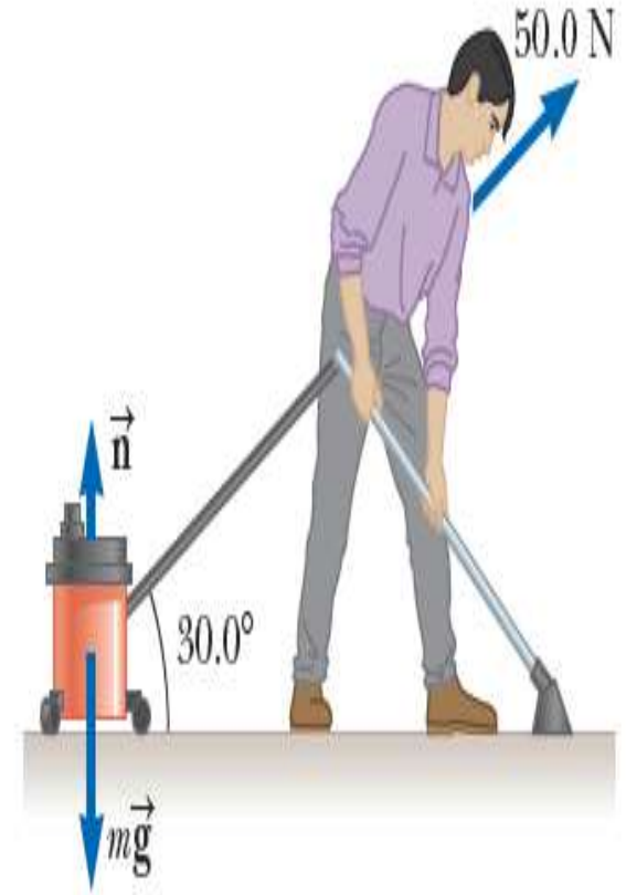
Figure 7.5: A vacuum cleaner being pulled at an angle of 30^\circ from the horizontal
